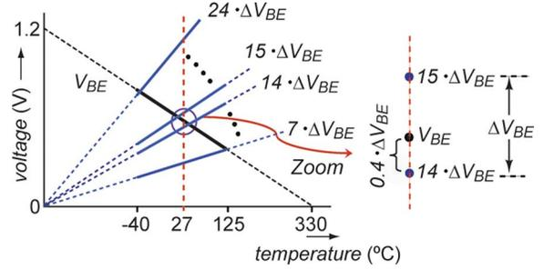
Fig. 7. Temperature dependence of  $k \cdot \Delta V_{BE}$  and  $V_{BE}$  from  $-40^\circ\text{C}$  to  $125^\circ\text{C}$ , e.g. at room temperature:  $14 \cdot \Delta V_{BE} < V_{BE} < 15 \cdot \Delta V_{BE}$ .
