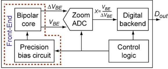
Fig. 3. Block diagram of the smart temperature sensor.
