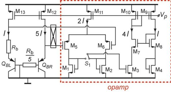
Fig. 6. Simplified circuit diagram of the bias current circuit (left hand side) and positive feedback opamp.
