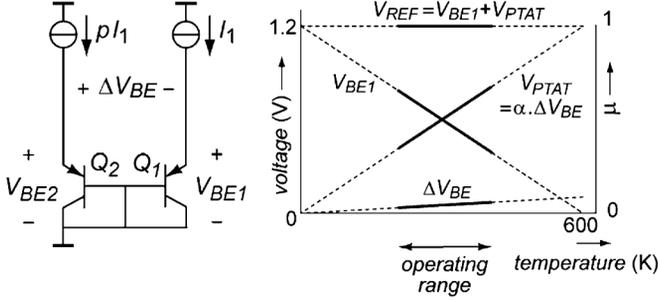
Fig. 1. Two substrate PNPs generate the required voltages ( $V_{PTAT}$  and  $V_{REF}$ ) for a ratiometric temperature measurement.
