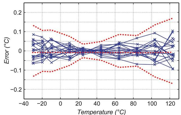
Fig. 16. Measured temperature error of 19 sensors after digital trimming at 25°C; dashed lines refer to the average and  $\pm 3\sigma$  limits.
