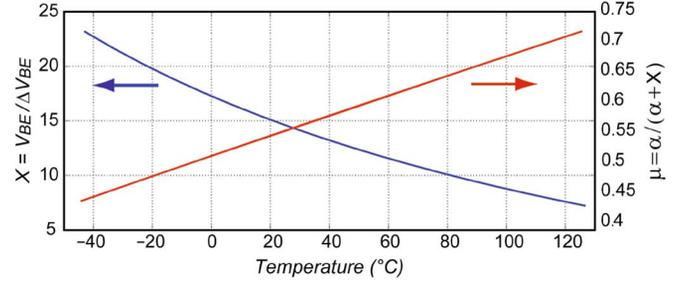
Fig. 2. Nonlinear  $X = V_{BE}/\Delta V_{BE}$  ( $p = 5$ ) and linearized  $\mu = \alpha/(\alpha + X)$  as a function of temperature.
