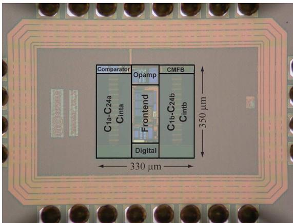
Fig. 14. Chip micrograph of the sensor.
