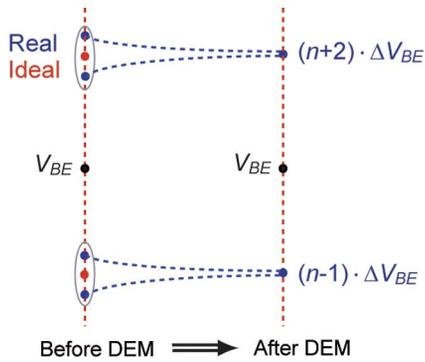
Fig. 13. Dynamic element matching of capacitors is used to enhance the accuracy of references during the fine conversion step.
