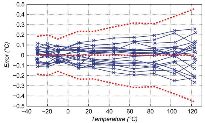
Fig. 15. Measured temperature error of 19 sensors before trimming; dashed lines refer to the average and  $\pm 3\sigma$  limits.
