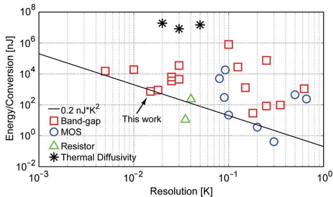
Fig. 17. Energy per conversion versus resolution for different smart temperature sensors using different sensing principles [19].
