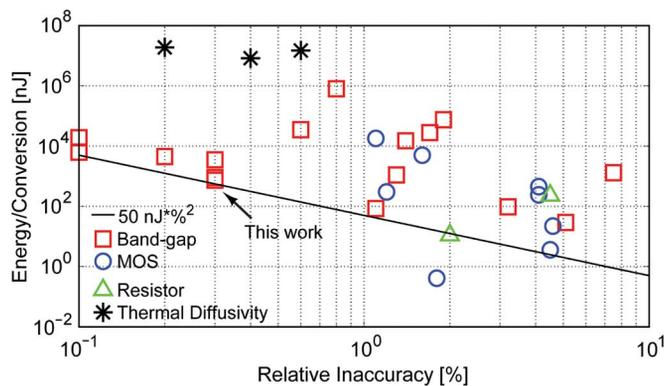
Fig. 18. Energy per conversion versus relative inaccuracy for different smart temperature sensors using different sensing principles [19].
