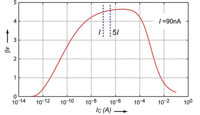
Fig. 5. The forward current gain  $\beta_F$  (at  $25^\circ\text{C}$ ) of a substrate PNP transistor ( $5 \mu\text{m} \times 5 \mu\text{m}$ ) as a function of collector current  $I_C$  in the 0.16  $\mu\text{m}$  CMOS process used.
