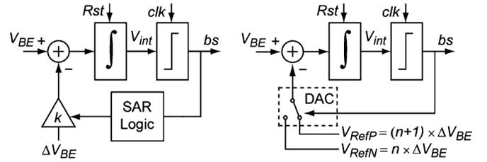
Fig. 8. Block diagram of the zoom ADC during the coarse (left) and fine (right) conversions.
