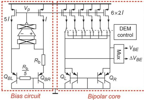
Fig. 4. Circuit diagram of the analog front-end.
