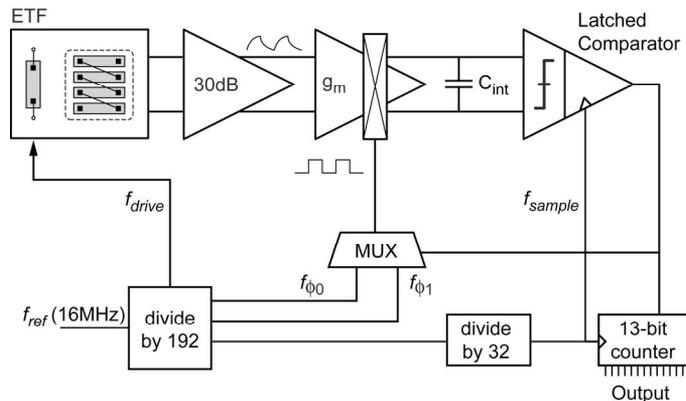
Figure 32.1.4: Block diagram of the PD $\Delta\Sigma$ M.
