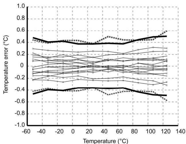
Figure 32.1.6: Measured temperature spread for 16 samples with  $P_{heat} = 2.5mW$ . Also shown are the  $\pm 3\sigma$  values (bold line:  $P_{heat} = 2.5mW$ , dashed line:  $P_{heat} = 1mW$ ).
