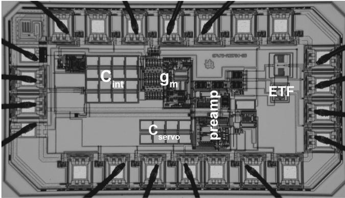
Figure 32.1.7: Chip micrograph of the ETF and the PD $\Delta$  $\Sigma$ M.
