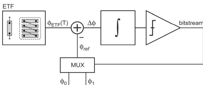
Figure 32.1.3: Block diagram of a phase-domain delta-sigma modulator (PD $\Delta\Sigma$ M), which digitizes the phase shift  $\phi_{ETF}$  of an ETF.
