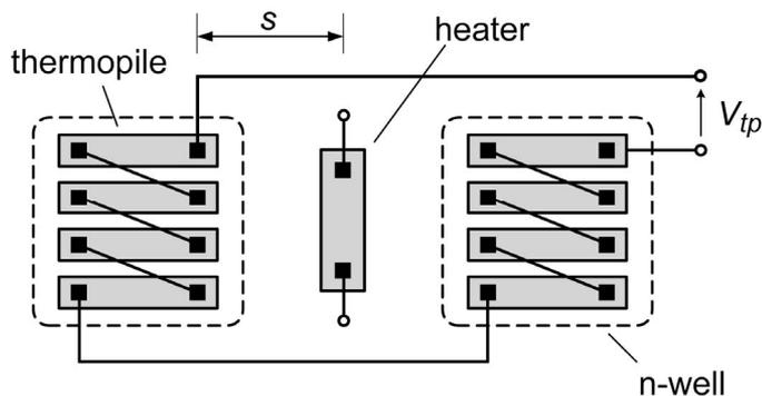
Figure 32.1.1: Schematic layout of an electrothermal filter (ETF) [1].
