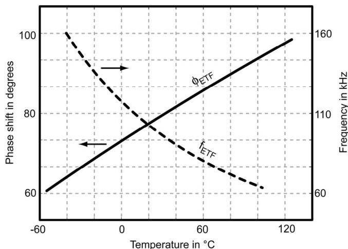
Figure 32.1.2: Simulated ETF output characteristics for both phase and frequency readout modes.
