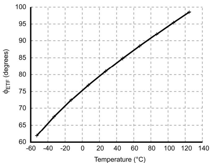
Figure 32.1.5: Measured ETF phase shift over temperature.
